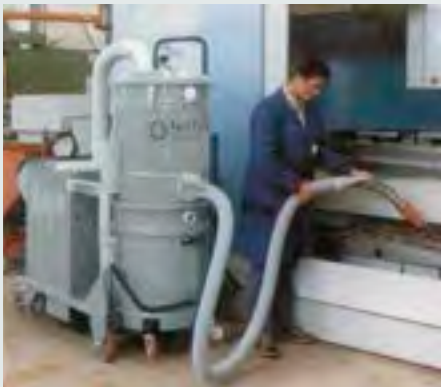
Metal sector: collection of shavings on machine tool
