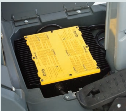
An integrated on-board charger enables easy plug-in and battery charge at any outlet
