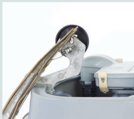
Built-in squeegee hanging system on recovery tank for easy machine transfer in narrow areas
