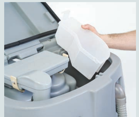
A debris tray captures the dirt from the suction hose to prevent it from entering the recovery tank
