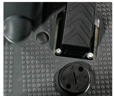
Fully adjustable traction pedal can be aligned with the operators choice of driving position
