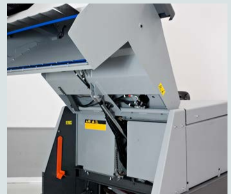
The CR 1500 can dump debris at a height of 152 cm
