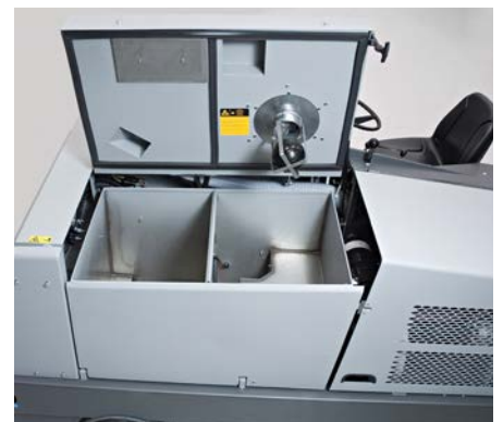
The recovery and solution tanks are squared and made of stainless steel. This allows them to be easily cleaned and it enables the use of hot water for better floor cleaning
