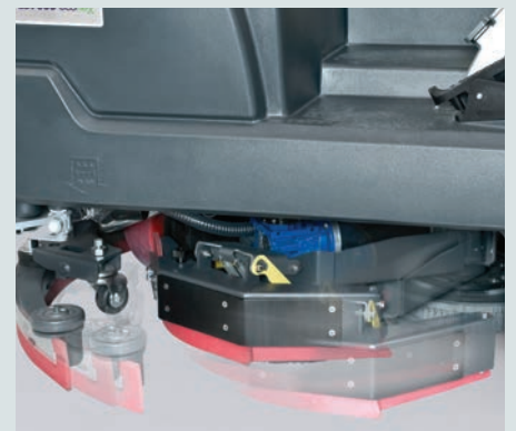
Pivoting off-set scrub deck and break-away squeegee won't be damaged if knocked by obstacles
