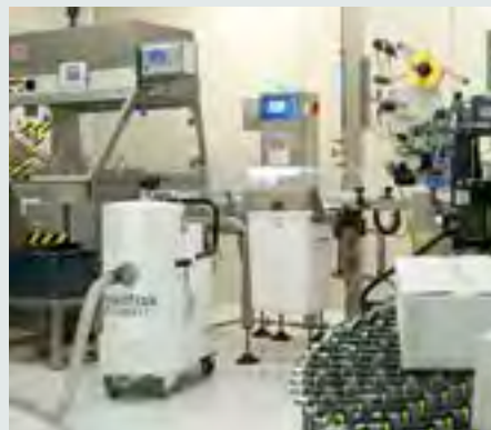
Recovery of waste from a packaging machine
