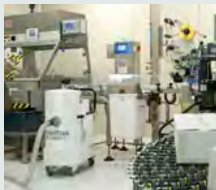
Recovery of waste from a packaging machine
